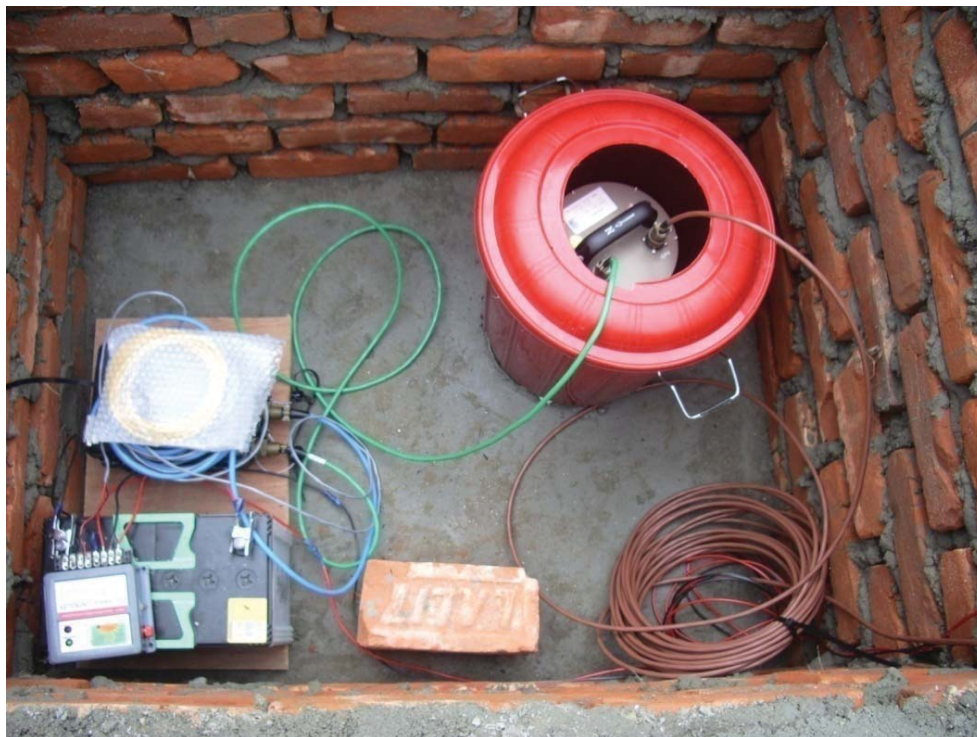
Fig. 15. Seismometer in the vault.
